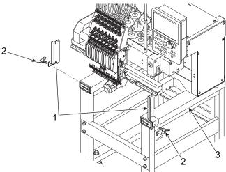
(2) Detach the box cover 4, and attach the screw 5 (hexagon socket head cap screw M5\*10) to the stand 3. Head part (tip) of the screw 5 is for positioning the table support base 6. At this time, attach the screw 5 to any position.
