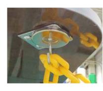
(14)Attach the magnet hanger to the main body of the machine, and hang the chain on it.
