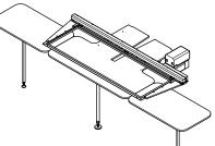
(10)Set the center table support and the (11)Fix the side table support by using knobbed screws.
